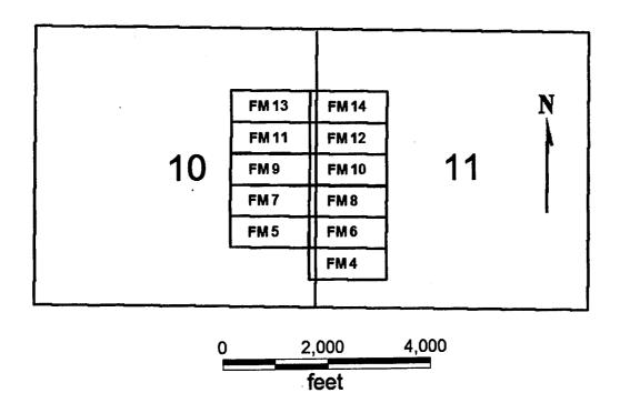
FM 4-14 All claims are 1500 x 600 Sides are E-W and ends are N-S All locations, corners and end centers are 5' 2x2 wood posts with metal tags
