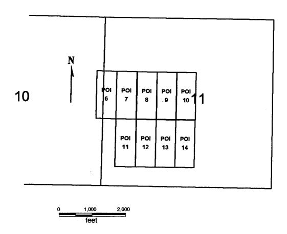
POI 6-14 All claims are 1500 x 600 Sides are N-S and ends are E-W All locations, corners and end centers are 5' 2x2 wood posts with metal tags
