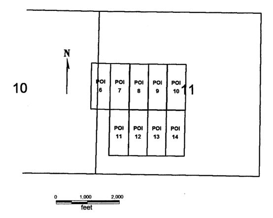
All claims are 1500 x 600 **POI 6-14** Sides are N-S and ends are E-W All locations, corners and end centers are 5' 2x2 wood posts with metal tags
