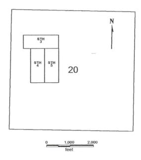
STH 3-5 All claims are 1500 x 600 Sides of 4 and 5 are N-S and ends are E-W, Sides of 1 are E-W with N-S sides All locations, corners and end centers are 5' 2x2 wood posts with metal tags
