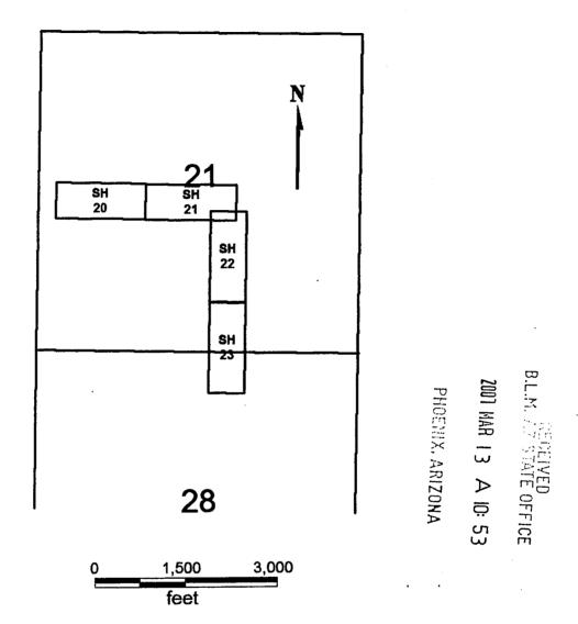
SH 20-23 All claims are  $1500 \times 600$  Sides of SH 20 and 21 are E-W, and sides of SH 22 and 23 are N-S. All locations, corners and end centers are 5' 2x2 wood posts with metal tags
