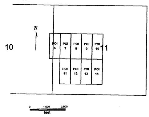
POI 6-14 All claims are 1500 x 600 Sides are N-S and ends are E-W All locations, corners and end centers are 5' 2x2 wood posts with metal tags
