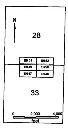
EH 47-52 All claims are 1500 x 600 Sides are E-W and ends are N-S All locations, corners and end centers are 5' 2x2 wood posts with metal tags
