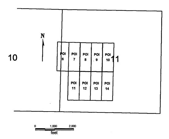
**POI 6-14** All claims are  $1500 \times 600$  Sides are N-S and ends are E-W All locations, corners and end centers are 5' 2x2 wood posts with metal tags
