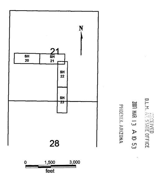
SH 20-23 All claims are 1500 x 600 Sides of SH 20 and 21 are E-W, and sides of SH 22 and 23 are N-S. All locations, corners and end centers are 5' 2x2 wood posts with metal tags
